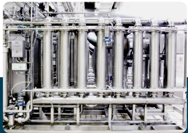
Typical filter block with 20 membrane inserts split in 4 clusters
