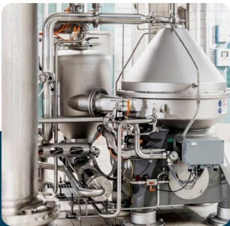
Typical centrifuge for pre clarification upstream filtration for 400 hl/h performance
