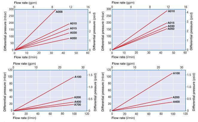
$^3$  For liquids with viscosities differing from water, multiply the pressure drop by the viscosity in cP.
