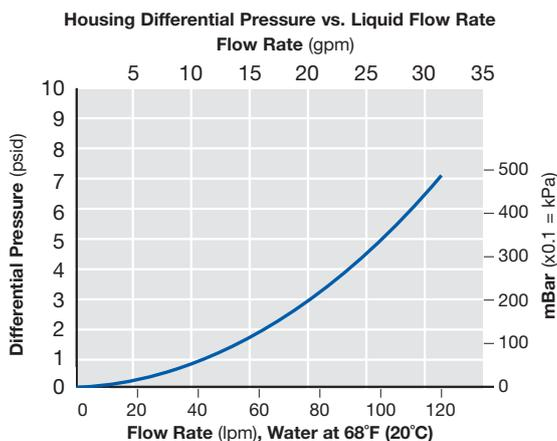
For liquids other than water, multiply differential pressure by specific gravity.
