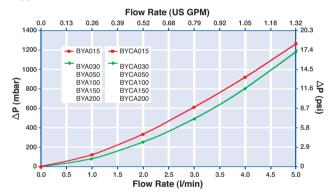
Por fluids of 1 cP viscosity. As a general guide, for other viscosities, multiply differential pressure by viscosity in cP.
