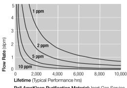
Pall AresKleen Purification Material: Inert Gas Service Gaskleen ST Purifier Assembly, Part # GLP5INPVMM4
