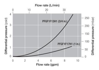
$<sup>^{\</sup>rm 3}$  For liquids other than water, multiply the pressure drop by the specific gravity of the fluid.
