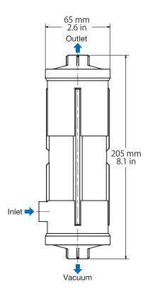
For best performance module should be installed vertically. Please review document number IUDM6EN for proper installation instruction. Document is available on the web at microelectronics.pall.com. For use in other configurations/flow patterns please contact the factory for assistance.
